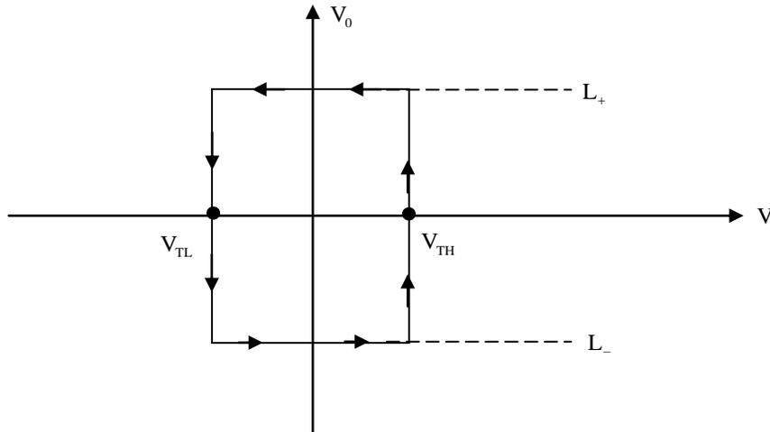
$$\begin{aligned} \text{Hysteresis} &= V_{TH} - V_{TL} \\ &= -L_- \left( \frac{R_1}{R_2} \right) + L_+ \left( \frac{R_1}{R_2} \right) \\ 500\text{mV} &= -(-5) \left( \frac{R_1}{20\text{k}} \right) + 5 \left( \frac{R_1}{20\text{k}} \right) \\ &= \frac{R_1}{2\text{k}} \end{aligned}$$
