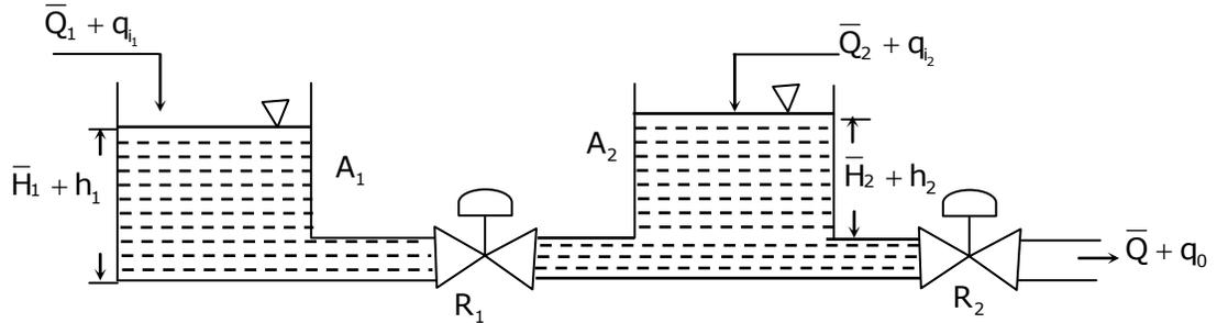
The liquid levels in the tanks may be assumed as output. Also draw the block diagram and obtain transfer function  $H_2(s) / Q_{i_1}(s)$  for transient state.
