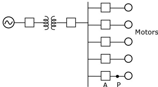
A 20 MVA 11 KV generator with  $X_d'' = 15\%$  is connected through a transformer to a bus which supplies five identical motors as given above.
