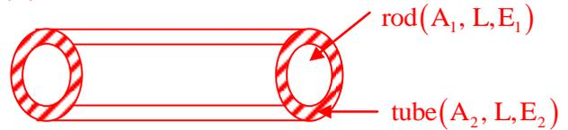
Assume  $P_1$  is the load applied on rod and  $P_2$  is applied on tube.
