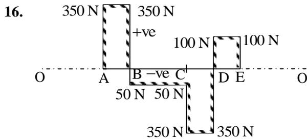
The shear force diagram of a single overhanging beam is shown in figure. One simple support is at end A. The 'total' downward load acting on the beam is
