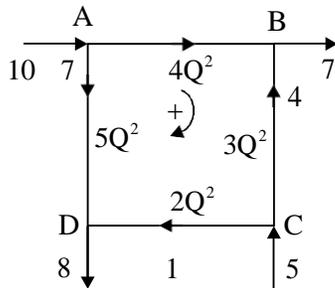
A pipe network is shown with all needful input data to compute the first iteration improved magnitudes of the initially assumed flows in the branches. What will be the such improved flow magnitudes in branches AB and CD? Consider to first decimal accuracy.
