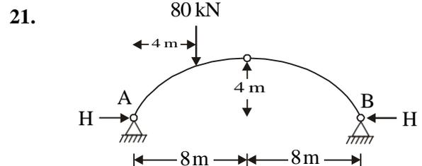
The horizontal thrust of the three-hinged arch loaded as shown in the figure is
