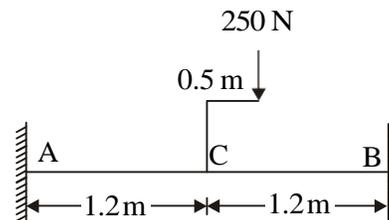
A horizontal, bar of 40 mm diameter solid section is 2.40 m long and is rigidly held at both ends so that no angular rotation occurs axially or circumferentially at the ends (as shown in figure). The maximum tensile stress in the bar is nearly
