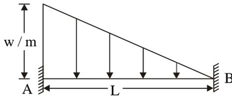
A fixed beam is loaded as in figure. The fixed end moment at support A is
