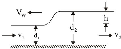
Consider the occurrence of a surge at the water surface of a wide rectangular channel flow, as in the figure, where the one-dimensionally considered velocities are  $v_1$  and  $v_2$  and the depths are  $d_1$  and  $d_2$ , with the surge height  $h$ , whereby  $d_2 - d_1 = h$ , moving at a speed of  $V_w$  over depth  $d_1$ . Joint application of continuity and momentum principles will indicate the surge front speed  $V_w$ , to be
