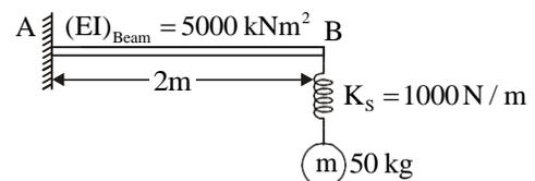
The fundamental time period of vibration of the system shown in the figure, by neglecting the self weight of the beam, is nearly
